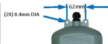
Hanger Removal & Mount Dimensions
